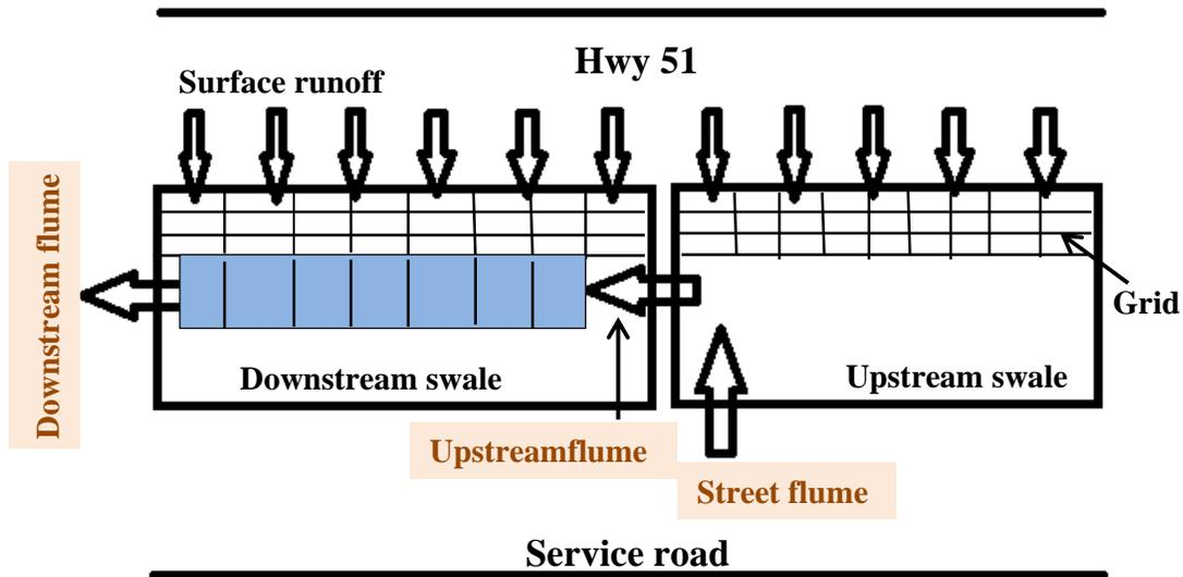
Figure 2. Plan view of the swale located near Hwy 51, Madison, WI.
